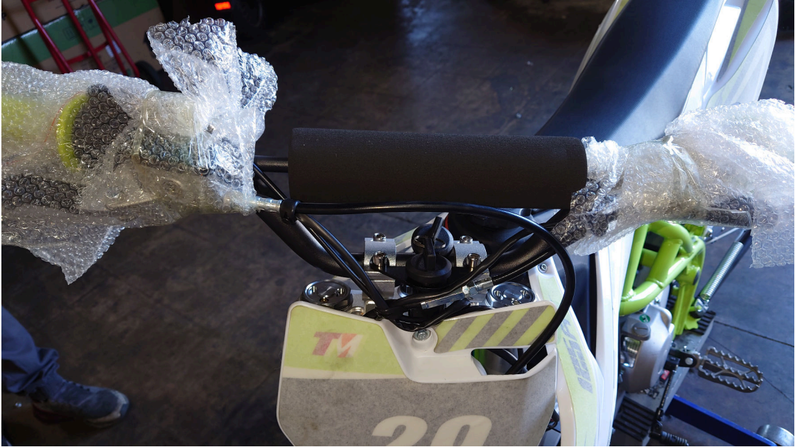
Figure 2.17.: Put on the Buffer Foam
