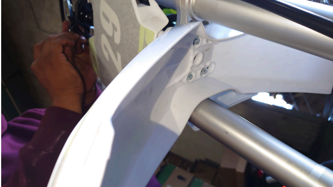
Figure 2.14.: Install the Front Fender
