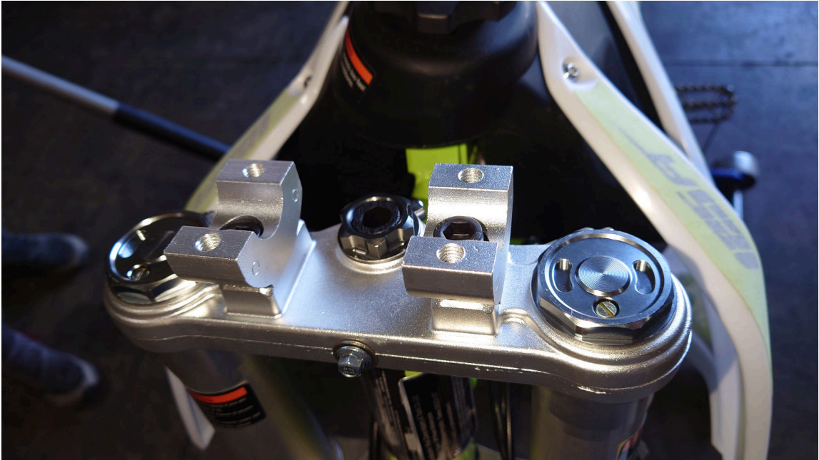
Figure 2.5.: Set up the Handlebar Supports
