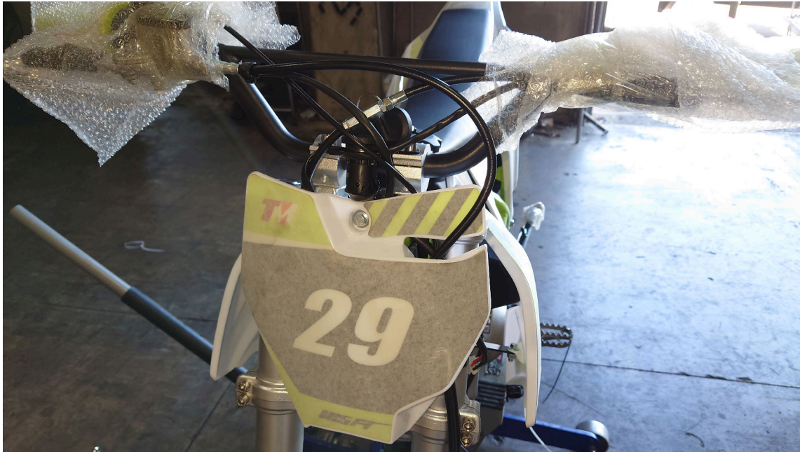
Figure 2.12.: Install the Number Plate
