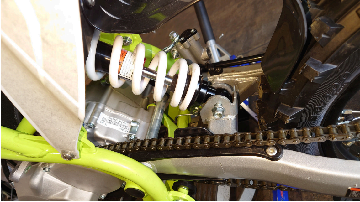
Figure 2.15.: Install the Rear Shock
