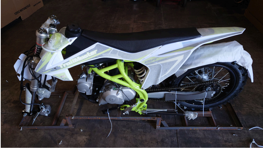
Figure 2.2.: Remove the Front Wheel, Accessories Box and Steel Fram
