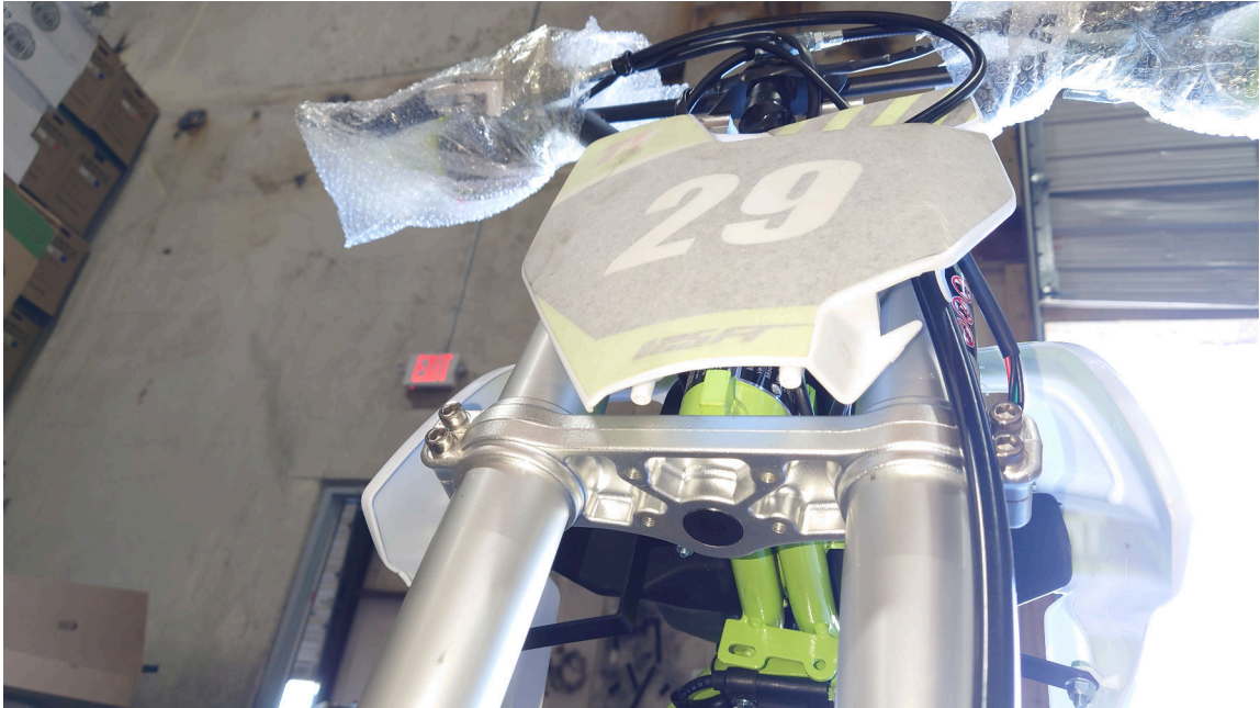
Figure 2.13.: Take off the Screws underneath the Triple Tree Clamp
