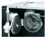
Kjeldahl etc. The Laboratory Mill 3100 is a hammer type cyclone mill, built into a soundproof casing. An adjustable vacuum feed control regulates the feed rate of the sample into a metallic grinding chamber. A hardened steel hammer rotates at high speed forcing the sample through a stainless sieve. Standard sieve of 0.8 mm is used for Falling Number, Glutomatic System and NIR analyses. Sieves from 0.5 – 2.0 mm are available. The fine, homogeneous sample is separated from air in a cyclone and
