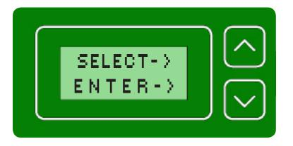
Once in the setup menu, the UP button will cycle through two setup options. Pressing the DOWN button will enter the selected function.
