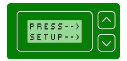
Turn on the power switch. When prompted, press the UP/DOWN buttons simultaneously to enter the set up menu.
