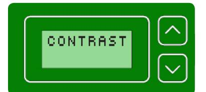
The contrast of the LCD character display can be adjusted between sixteen levels. With Contrast selected, press the DOWN Button to enter the function. Use the UP/DOWN buttons to adjust the contrast. Once the desired Contrast level is set, press the START Button to save the changes and exit.
