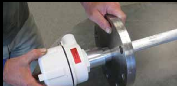
The rotary can then be mounted by screwing it into the coupling or mounting plate.
