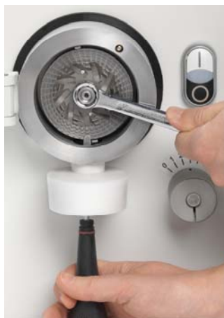
Figure 7. Loosening the center nut. Figure 8. Pulling out the disc. Figure 9. Position of stationary disc.
