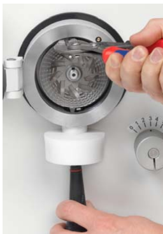
Figure 7. Loosening the center nut. Figure 8. Pulling out the disc. Figure 9. Position of stationary disc.
