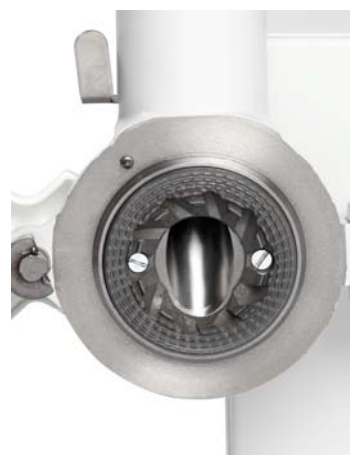
Figure 7. Loosening the center nut. Figure 8. Pulling out the disc. Figure 9. Position of stationary disc.
