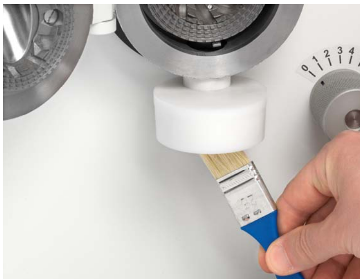
Figure 6. Cleaning of the milling chamber outlet.
