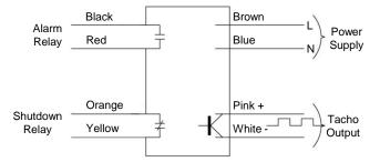
The diagram shows the state of the internal contacts with power applied. See installation manual for wiring procedure. The unit can be used with or without the tacho output.
