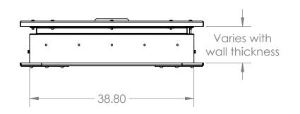
Rhino Metals Inswing Door 82" H x 40" W Minimum Rough Opening 82.75" H x 39.5" W Maximum Rough Opening 83" H x 41" W Minimum Wall Thickness
