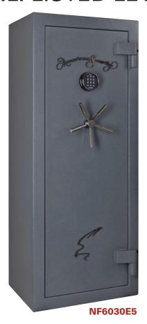
The American Security Products NF Gun Safe offers both superior performance and value. For burglary protection, it has a stout 1/4"-thick steel plate door. For fire protection, it is lined with 3 to 4 layers of drywall that are strategically engineered for optimal fire protection. This enables the NF Gun Safe to pass a verified 90-minute fire test at Intertek, an independent testing laboratory.
