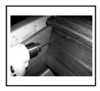
16.) Install the console shelf to the inside of the middle console leg and inside of the starboard seat clamp using #8 X 1 1/2" flat head screws. Using the same screws, fasten the instrument panel to cover the rectangle hole on the left side dash of the console.
