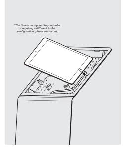
6 Install the tablet and the tablet power cable.
