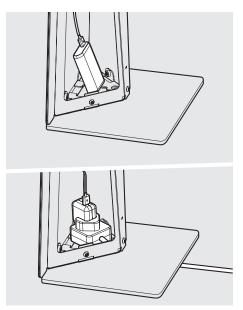
Connect the tablet cable to a power source.
