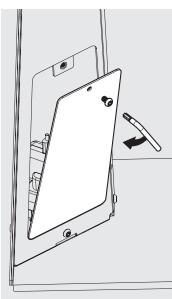
Locate and secure the Access Panel to the Mounting Arm.
