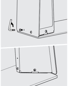
Secure the Mounting Arm to the Mount Bracket, with 5x M6x10mm screws.
