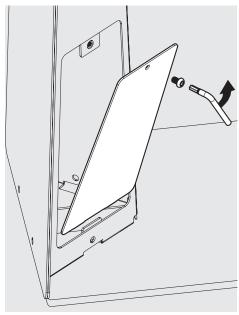
Remove the Mounting Arm Access Panel. Safely store this aside for use
