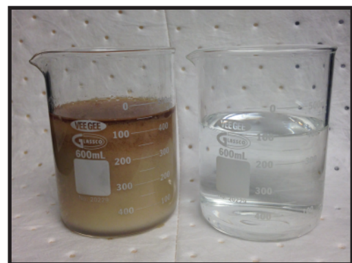
Oily Wastewater prior to Ultrafiltration (left) Filtered Oily Wastewater after Ultrafiltration (right)
