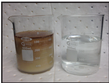
Oily Wastewater prior to Ultrafiltration (left) Filtered Oily Wastewater after Ultrafiltration (right)
