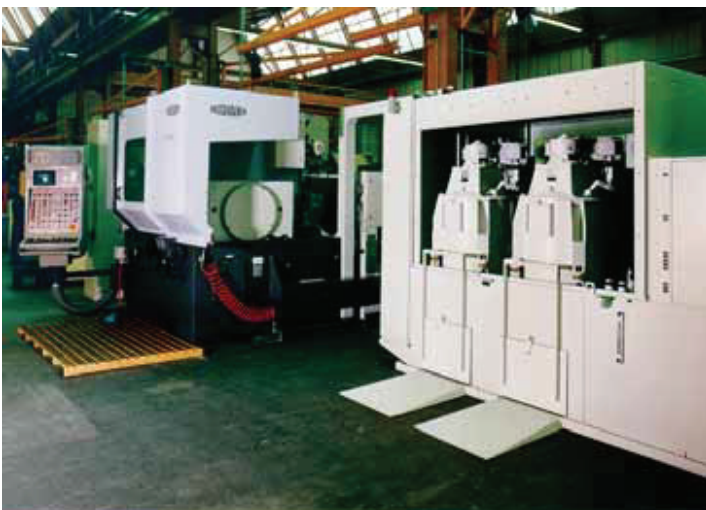
Dual T40 Automatic Discharging Centrifuge with a processing rate of 80 GPM
