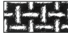
Monofilament Mesh is woven from single-fiber threads. The openings are square and uniform. Bags made from this material have excellent strength.
