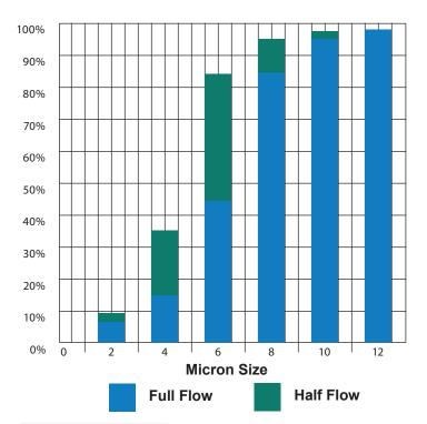
Most Centrifuge manufacturers provide average removal efficiencies based on the G Force and dwell time of the centrifuge of spherical Steel particles in water. The 1,800 rpm LiquaPac will remove approximately 95% of the solids above 8 micron at 15 gpm. The 2,500 rpm LiquaPac can remove about 98% of the solids above 5 micron at 15 gpm.
