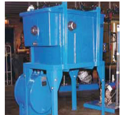
Optional elevated stand discharges oil directly into a reservoir
