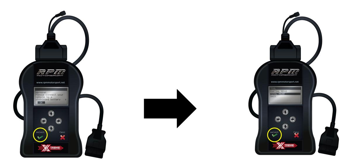
Note: The "Total Read" may take up to 1 hour to complete. A Total Read is only required if you have already done a Partial Read and sent your file to Rpm Motorsport and we have informed you that a Total Read is necessary.
