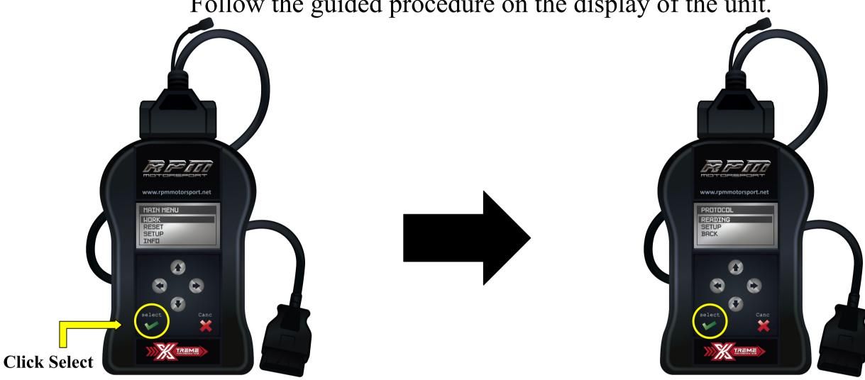
C) After the correct identification of the protocol proceed with the reading (or identification only) of the software stored in the vehicle ECU/DME, always following the guided procedure on the display of the unit.
