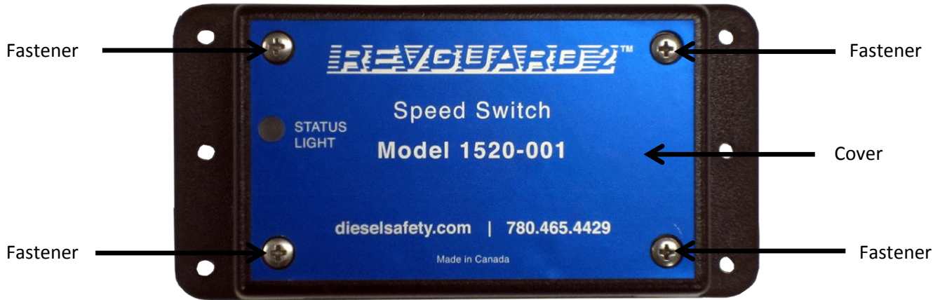
Figure 1: The Revguard 2 module lies underneath the blue cover.
