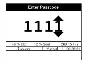
The passcode will be entered left to right. Utilize the up and down arrows, and press the Enter button after each correct number. If you enter the wrong passcode, it will reset the display to 0000, allowing you to restart the entry process.
