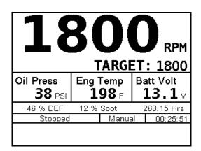
The main screen (shown above) displays actual and target RPM, Oil Pressure, Engine Temperature, Battery Voltage, Engine Hours, Engine State and Mode of Operation.
