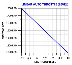
**NOTE:** In order for linear auto throttle to work correctly the auto start/stop function and auto throttle method need to be set to the same transducer type.
