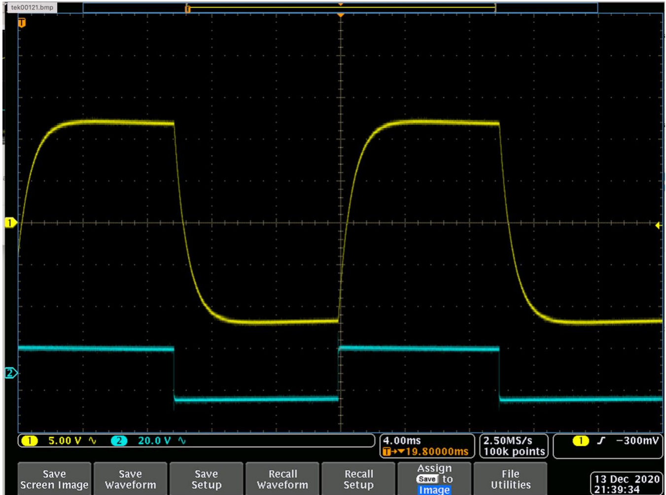
Depiction of 50 Hz PWM using no Dither. Lower waveform is voltage, upper waveform is the signal passed through a low pass filter (note no Dither present).
