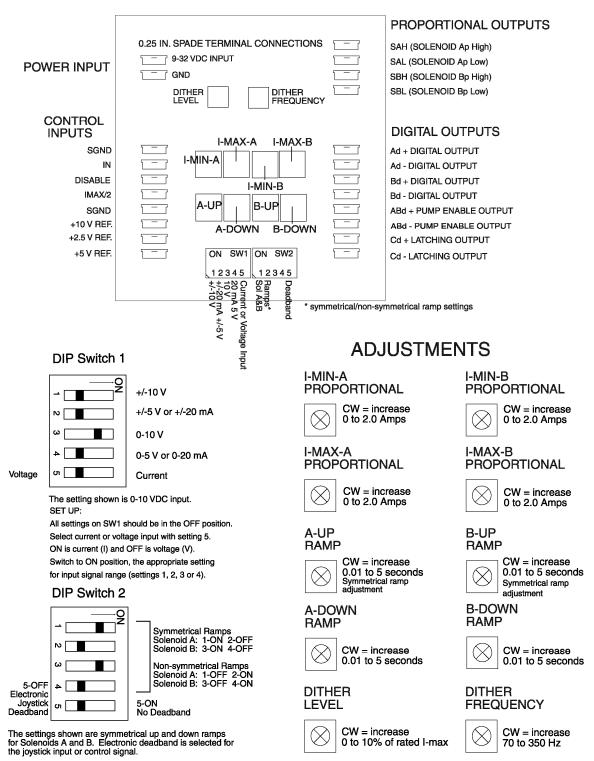
Adjustments to the single turn potentiometers are made using a flat head or Philips screwdriver. For P/N: DSDA-SMB-SC-MT-1A, minimum and maximum current adjustments are 20 turn pots.
