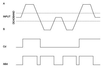
The Cd signal output turns on when the input signal reaches the +7.5 degree deadband setpoint. It remains on until the input signal reaches the -7.5 degree deadband setpoint (opposite direction).
