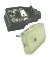
**Function:** The connector amplifier supplies a solenoid valve with current proportional to an input control (voltage, 0-20mA, potentiometer or pre-set level).
