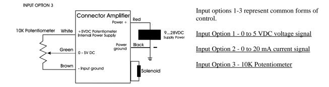
Another input option is **soft shift control**. This form of control permits gentle acceleration of the valve while using minimal external components. No control knobs are required.
