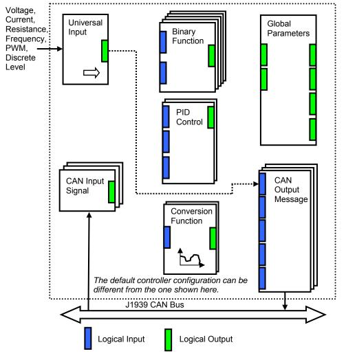
As an example, the logical output of the Universal Input functional block is connected to the logical input of the CAN Output Message functional block, providing a direct path for the input signal to the controller CAN output.
