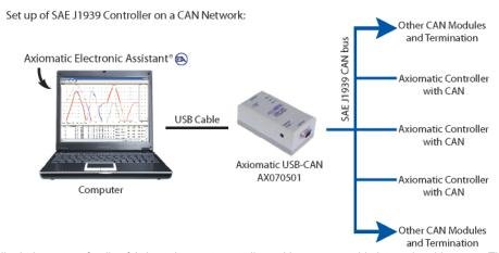
The controller belongs to a family of Axiomatic smart controllers with programmable internal architecture. This provides users with flexibility, allowing them to build their own custom controller with a required functionality from a set of predefined internal functional blocks using the PC-based Axiomatic Electronic Assistant® software tool. Application programming is performed through the CAN interface, without disconnecting the controller from the user's system.
