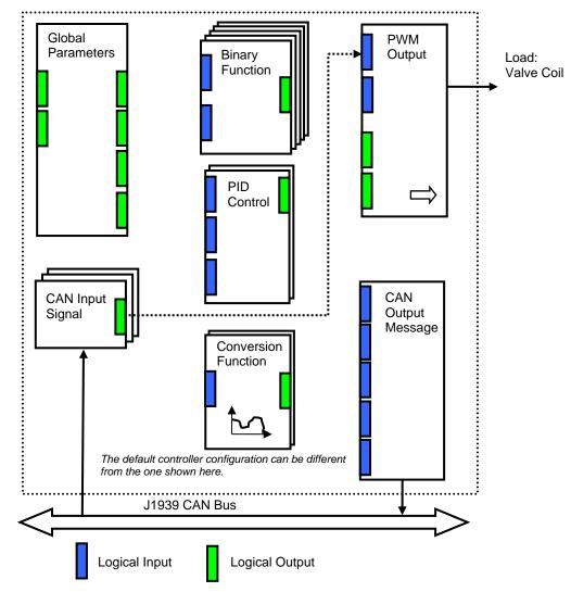
As an example, the logical output of the CAN Input Signal functional block is connected to the logical input of the PWM Output functional block, providing a direct path for the CAN input signal to the controller output.
