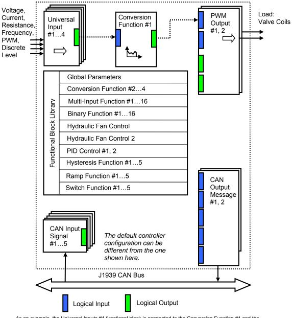
As an example, the Universal Inputs #1 functional block is connected to the Conversion Function #1 and the Conversion Function #1 is connected to the PWM Output #1 functional block, providing a path for the input signal from input to output through the Conversion Function #1 functional block.
