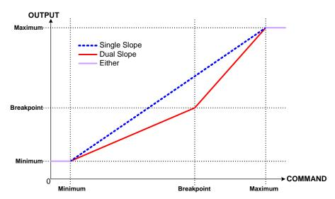
Figure 1 – Proportional Output vs. Command Profile
