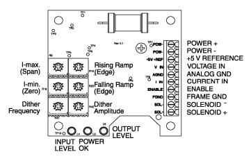
In the Packaged Driver, adjustments are accessible by loosening the four screws on the lid of the housing and removing the lid.
