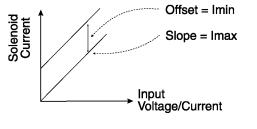
Adjusting the maximum current (I-max.) does not affect the minimum current (I-min.) setting.
