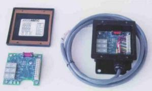
**Application:** Accurate control of hydraulic and pneumatic proportional solenoid valves used in mobile equipment and industrial processes.
