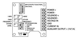
P/N: RSD-SMB-3A-00 is shown above without its metal housing. The PCB only model p/n: RSD-PCB-3A has the 8-pin connector reversed to permit wiring from the right hand side.
