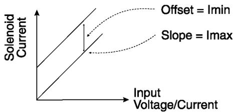
Adjusting the maximum current (I-max.) does not affect the minimum current (I-min.) setting.
