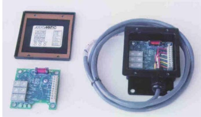
**Application:** Accurate control of hydraulic and pneumatic proportional solenoid valves used in mobile equipment and industrial processes.
