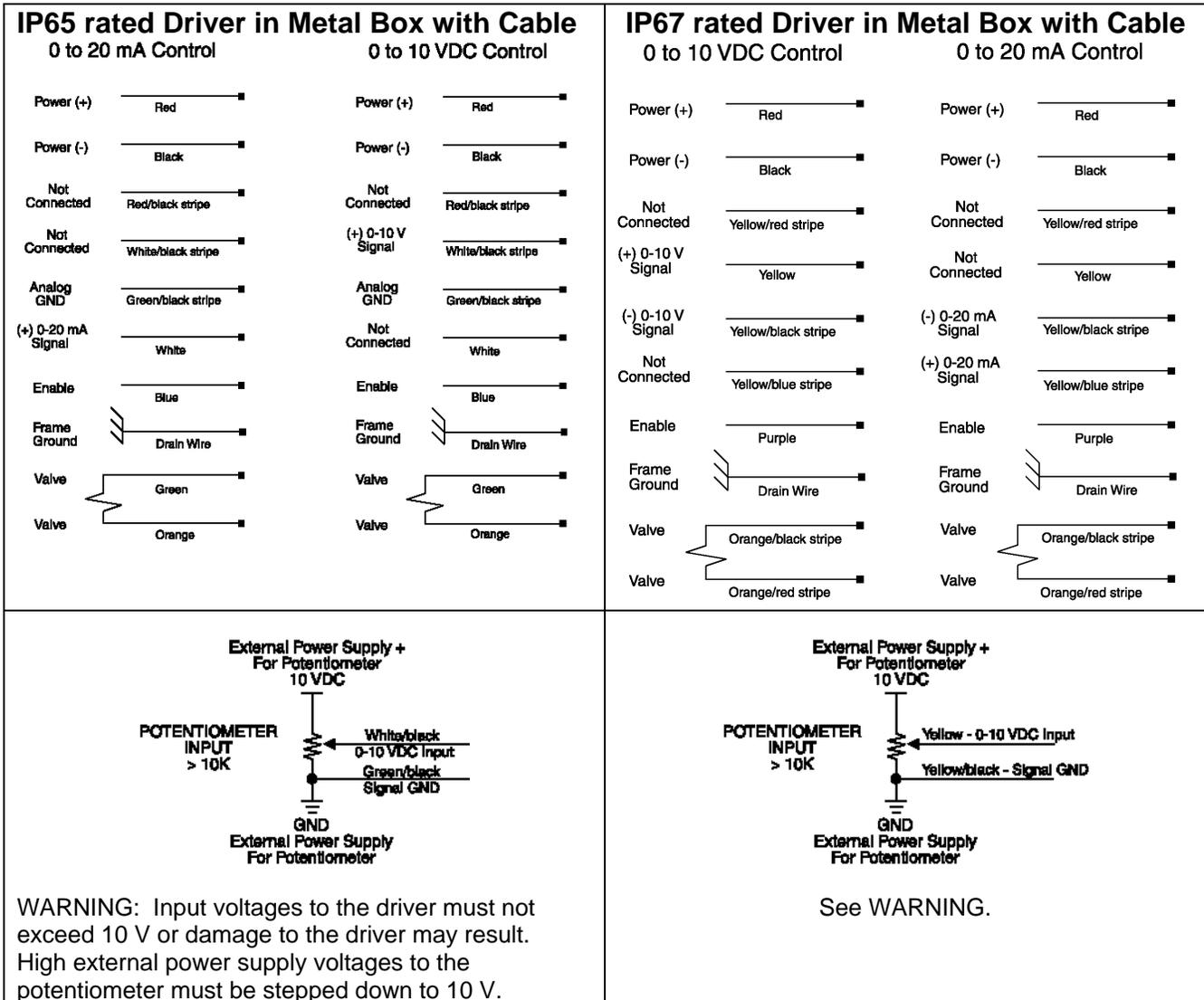
Refer to page 2 (block diagram) for an alternative method of connecting a current loop transmitter to provide a current control signal input. In this method, the current loop transmitter receives power from the power supply powering the amplifier. The transmitter is connected to the driver's +power supply input wire and the +0 to 20mA input wire. This method does not use the Analog GND wire connection.
