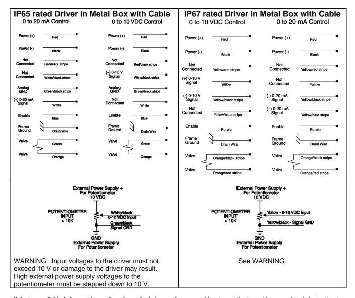
Refer to page 2 (block diagram) for an alternative method of connecting a current loop transmitter to provide a current control signal input. In this method, the current loop transmitter receives power from the power supply powering the amplifier. The transmitter is connected to the driver's +power supply input wire and the +0 to 20mA input wire. This method does not use the Analog GND wire connection.
