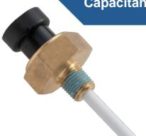
The level switch is an active device designed to give an alarm signal if liquid falls below, or rises above, a preset level. It can be specified with a delay to eliminate false alarms due to turbulence.
