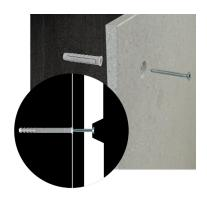
Our easy to use anchoring system can be used without tile cement. Contact us for more information on installing with anchors. Screw fastening is the most cost effective install method. Make sure to use thick foam spacers on anchor areas to make levelling process easier and in case walls are not level.
