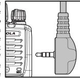
the plug using the screws supplied with the Speaker/ Microphone. Hold the speaker grille up next to your ear while receiving. To transmit, press the **PTT** switch on the Speaker/Microphone, just as you would on the main transceiver's body, and speak into the microphone on a normal voice level.
