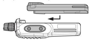
☐ To remove the battery, turn the radio off and remove any protective cases. Slide the Battery Pack Latch on the bottom of the radio toward the front panel while sliding the battery down about 1/2 inch (1.5 cm). Then lift the battery out from the radio.
