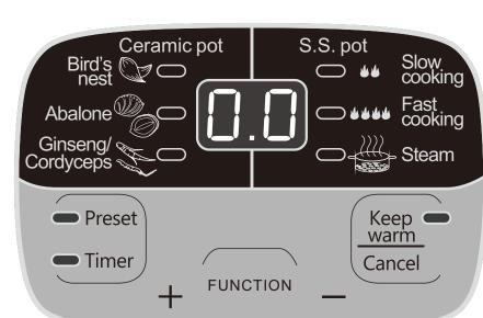
1. "Preset" key: On the standby mode, press the "Preset/Timer" key once, the presetting indicator and the screen displays "2.0" will flash alternately. At this moment, you can press the "+" "-" key to adjust the presetting time. Note: The presetting function means that the cooker will begin
