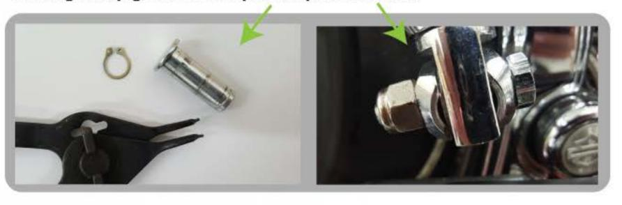
4. Slide footpeg mount into clevis with the wave spring and reinstall pin and clip or nut and bolt.
