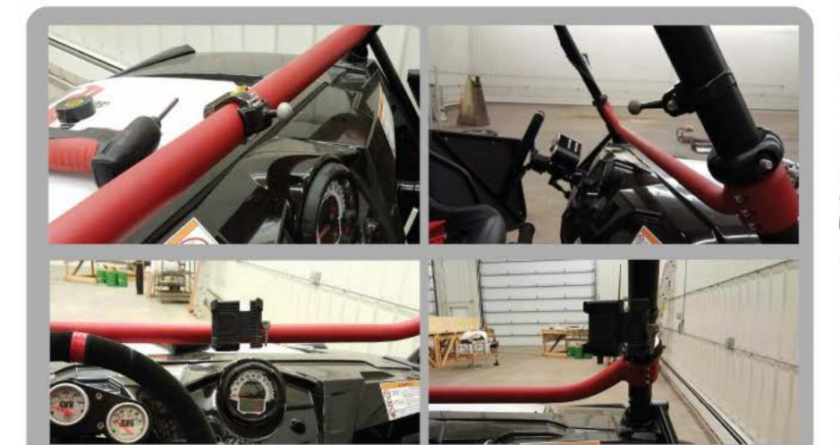
5. You may now mount any Ciro Ball Mount Accessory by simply snapping it on and tightening the nut.
