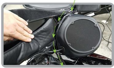
10. Plug supplied y adapters into already installed splitter harness, then plug wires from Tour Blade into y adapters, brown wire in line with brown and violet wire in line with violet. Use a small amount of dielectric grease on connectors. Turn on accessory power to verify that the light is functioning correctly.
