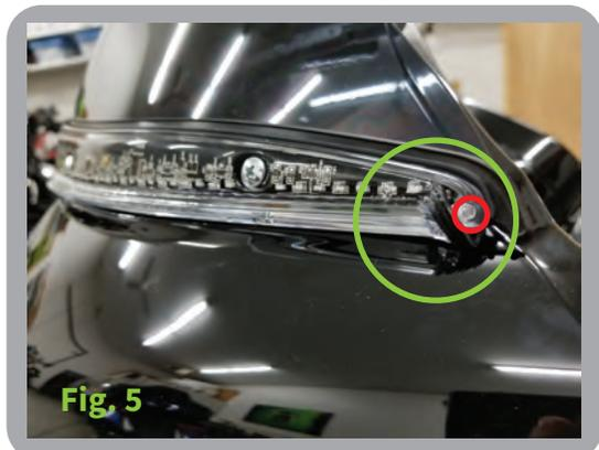
7. Route the wire as seen in Fig. 5 through the gap at the bottom of the lens. Make sure that the wire is out of the way of the screw you will be installing at the end of the trim. (Circled in red)
