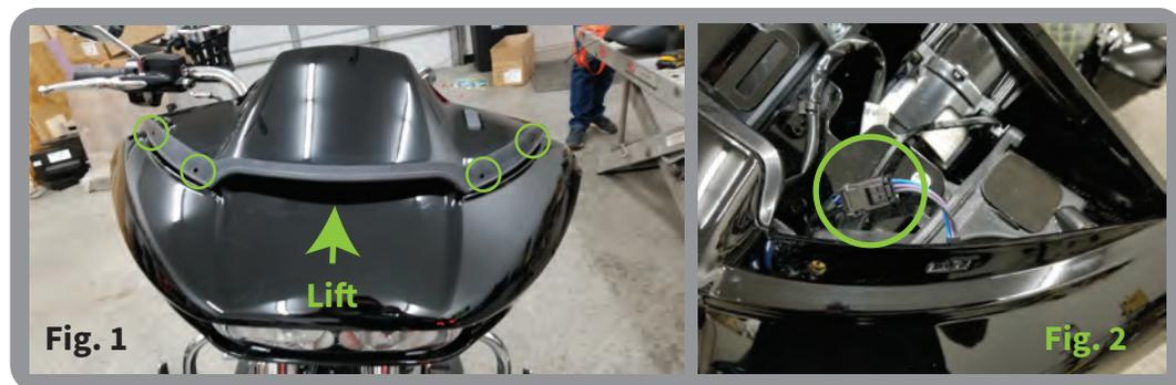
3. Locate the lighting plugs on both the left and right side of the fairing circled above. (Fig. 2)
