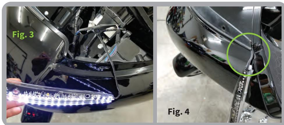
5. Re-install the plastic trim from step 2, with about an inch of wire for the lights routed out of the corner above the speaker as seen in Fig. 4.
