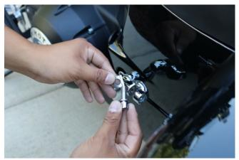
2. Place the spring washer into the female clevis of the comfort peg mount.
