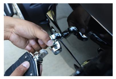
4. Insert the bolt and crush washer. Tighten appropriately.
