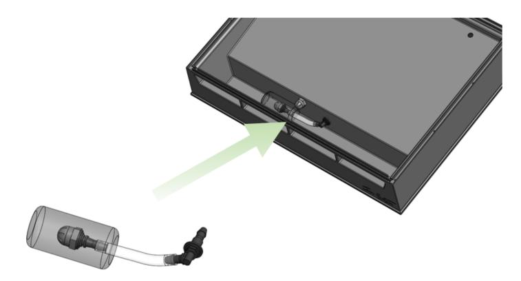
Figure 10 - Trough Inlet Assembly & Installation
