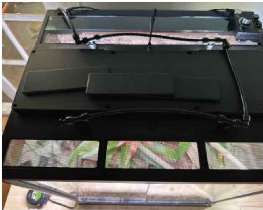
The hood supports three Mist King nozzles in the front and two in the rear.
