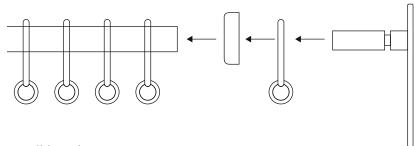
3. Slide the pole onto the wall bracket.
