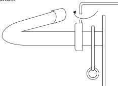
4. Tighten up the lock collar hex key using the key provided. The screw should go through the hole in the pole and lock into the wall bracket.
