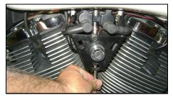
**3**-Disconnect the factory wiring from the coils & set the coil pack aside.
