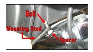
**6**-Slide the coils onto the mounting studs and install the washer and nut. Make sure to run the spark plug wire between the mounting studs before putting the coil on. Tighten valve cover bolts and coil mounting nuts. Don't over tighten.
