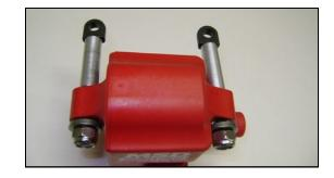
7-Install the spark plug wire onto each coil. Install the supplied wiring harness to each coil (long harness to the rear coil) and connect the other end back into the factory harness. Make sure to push all connectors until the lock snaps into place. NOTE: factory harness white wire and green stripe is the rear cylinder.
