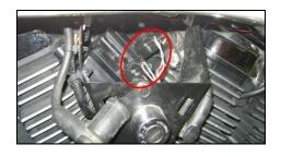
4-With a 5mm allen wrench remove the 2 valve cover bolts on each cylinder. (Removing the gas tank bolts and lifting it up a bit will help to gain easier access to the bolts but its not necessary. No matter how you do it, it's a pain in the butt!)
