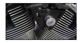
**2**-It is not necessary to remove the cheese wedge mount bracket & ignition key cylinder unless you plan on relocating the ignition. Disconnect the spark plug wires from the coils. With a long extension & 10 mm socket, reach up behind the ignition key cylinder and unscrew the bolt holding the coils to the mount.
