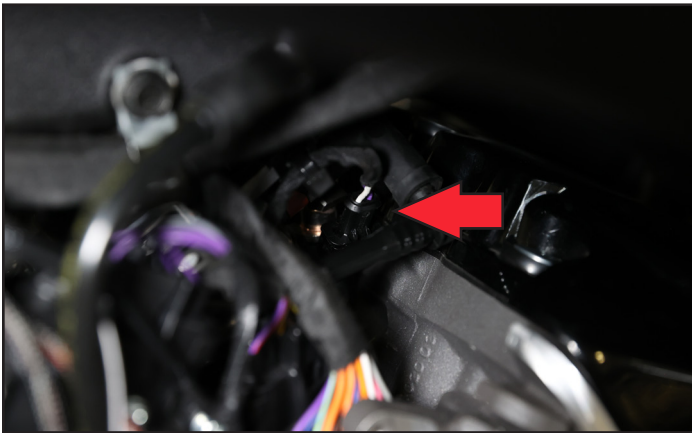
UNPLUG FRONT INJECTOR
