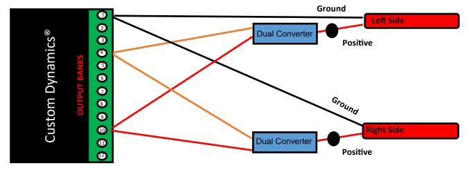
**Dual Converter** Orange—Running Light Red—Brake
