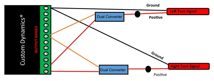
**Dual Converter** Orange—Running Light Red—Brake/Turn
