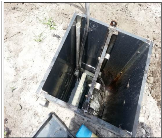
Figure 7 - Autosampler intake tube, conductivity, and temperature probe (left) prior to installation within IDT control box (right)
