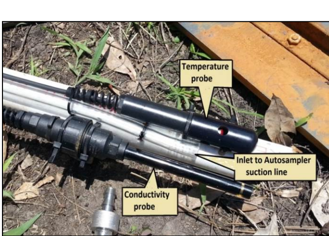
Figure 7 - Autosampler intake tube, conductivity, and temperature probe (left) prior to installation within IDT control box (right)
