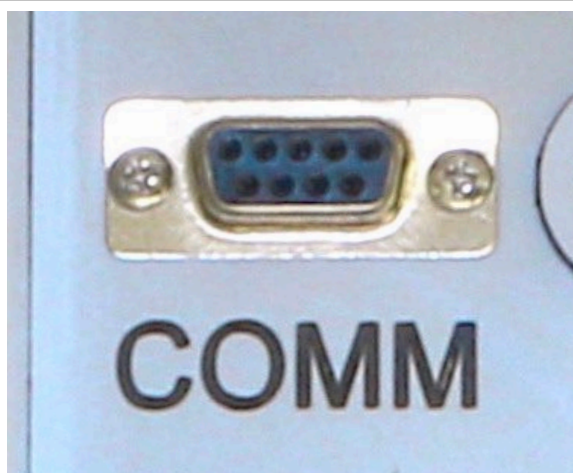
STEP 2. Connect COMM Cable to your monitor, and make sure the power is on
