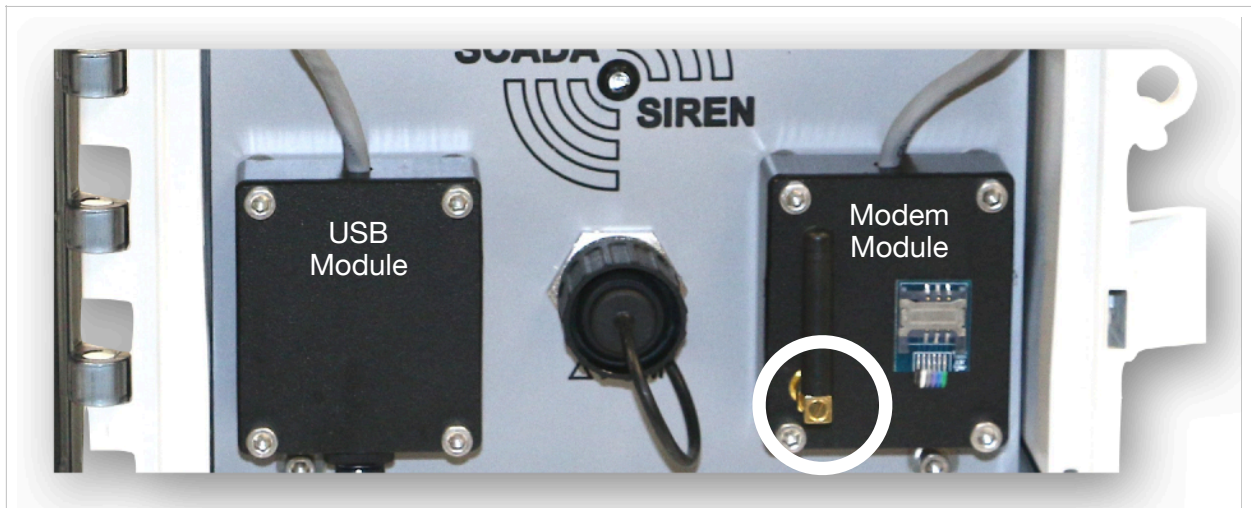
INSTALL SMA ANTENNA
