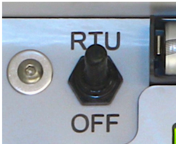
Turn the RTU Power ON by flipping the switch to the UP position
