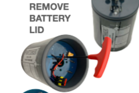
UNSCREW TWO HEX BOLTS REMOVE BATTERY CARD
