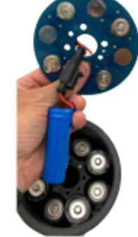
LOAD NEW BATTERIES WITH NEGATIVE SIDE TOWARDS SPRING and REASSEMBLE
