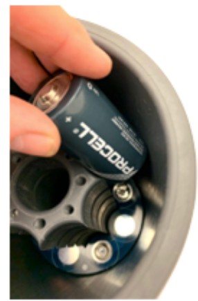
LOAD NEW BATTERIES WITH NEGATIVE SIDE TOWARDS SPRING and REASSEMBLE
