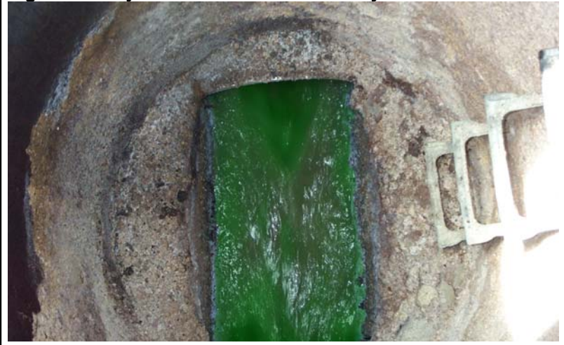
Figure 2.5. Dyed Water Visible in Sanitary Sewer
